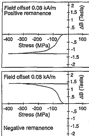
Figure 3. The variation in magnetic induction  $B$  with compressive applied stress under an applied field of  $H = 80 \text{ A m}^{-1}$  after Pitman [19]: (a) above the anhyseteric and (b) below the anhyseteric.
