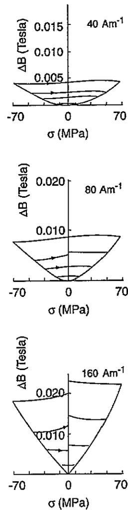
Figure 6. The variation in magnetic induction  $B$  with stress for Fe-0.2 wt% C as reported by Birss *et al* [9] at field strengths of 40, 80 and 160  $\text{A m}^{-1}$ .
