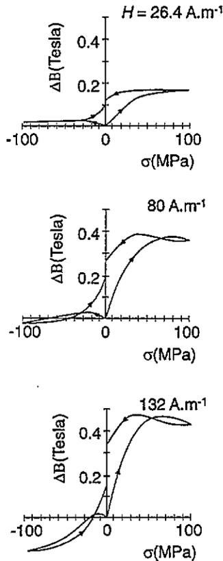
Figure 5. The variation in magnetic induction  $B$  with stress for mild steel as reported by Craik and Wood [8] at field strengths of 26, 80 and 132  $\text{A m}^{-1}$ .
