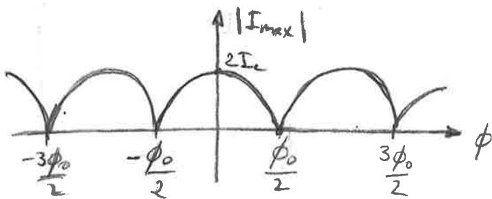
← the SQUID behaves as a single Josephson junction with critical current controlled by the magnetic flux.
