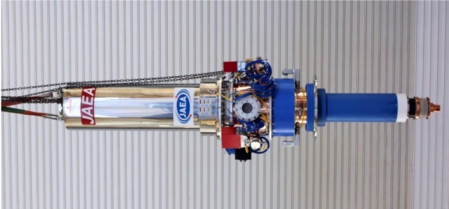
Each of ITER's 24 gyrotrons will generate a microwave beam over a thousand times more powerful than a traditional microwave oven. [www.iter.org](http://www.iter.org).
