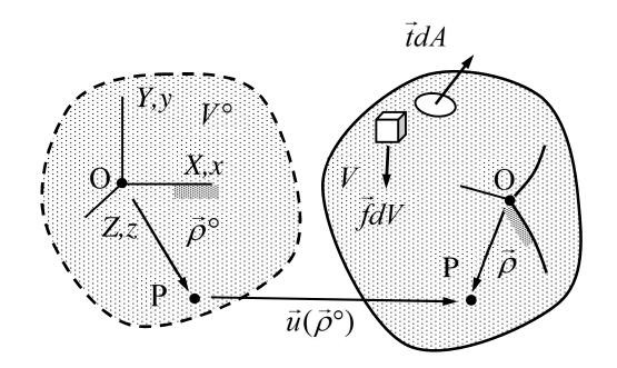
A constitutive equation  $f(\vec{\sigma}, \vec{u}) = 0$  brings the material details into the model. For an unique solution, a displacement boundary condition is needed somewhere on  $\partial V$ .
