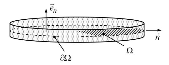
If the external forces on the top and bottom surfaces vanish and stress is symmetric 'a priori', virtual work expressions of the internal and external forces simplify to (volume element dV = dndA and area element on the boundary dA = dnds)
