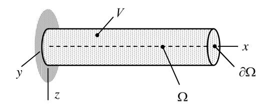
Let us consider the steps in the Cartesian (x, y, z) –coordinate system for clarity. The bar model assumes that displacement and stress have just axial components depending on the axial coordinate only. Representations of stress, displacement and gradient operator are  $\vec{\sigma} = \sigma_{xx}\vec{i}\vec{i}$  and  $\vec{u}(x) = u(x)\vec{i}$ ,  $\nabla = \vec{i}\partial/\partial x + \vec{j}\partial/\partial y + \vec{k}\partial/\partial z$
