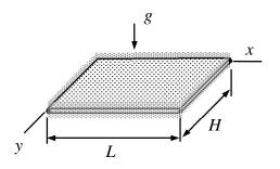
$$\delta W = -\int_{\Omega} \left\{ \begin{aligned} \frac{\partial^2 \delta w}{\partial x^2} \\ \frac{\partial^2 \delta w}{\partial y^2} \\ 2 \frac{\partial^2 \delta w}{\partial x \partial y} \end{aligned} \right\}^{\mathrm{T}} D \begin{bmatrix} 1 & v & 0 \\ v & 1 & 0 \\ 0 & 0 & \frac{1}{2}(1-v) \end{bmatrix} \begin{cases} \frac{\partial^2 w}{\partial x^2} \\ \frac{\partial^2 w}{\partial y^2} \\ 2 \frac{\partial^2 w}{\partial x \partial y} \end{cases} dA + \int_{\Omega} \delta w b_n dA \,.$$
