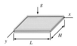
$$\delta W = -\int_{\Omega} \left\{ \begin{aligned} \frac{\partial^2 \delta w}{\partial x^2} \\ \frac{\partial^2 \delta w}{\partial y^2} \\ 2 \frac{\partial^2 \delta w}{\partial x \partial y} \end{aligned} \right\}^{\mathrm{T}} D \begin{bmatrix} 1 & v & 0 \\ v & 1 & 0 \\ 0 & 0 & \frac{1}{2}(1-v) \end{bmatrix} \begin{cases} \frac{\partial^2 w}{\partial x^2} \\ \frac{\partial^2 w}{\partial y^2} \\ 2 \frac{\partial^2 w}{\partial x \partial y} \end{cases} dA + \int_{\Omega} \delta w b_n dA \, .$$
