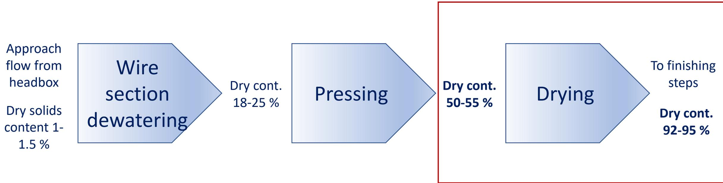
Drying is 300 times more expensive than dewatering in forming section
