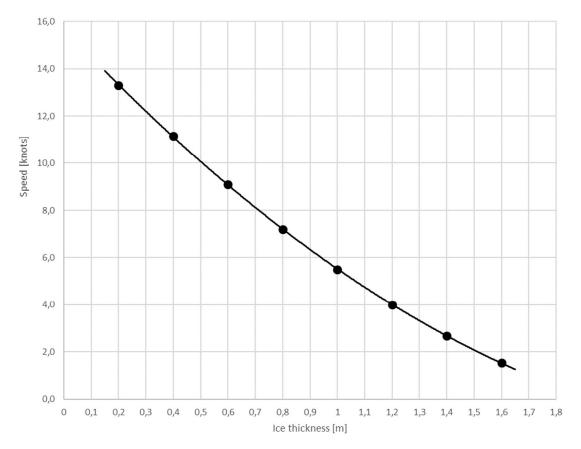
From the h-v-curve, we can read that the <u>vessel can achieve a speed of 10 knots in about 0.5 m</u> thick level ice.
