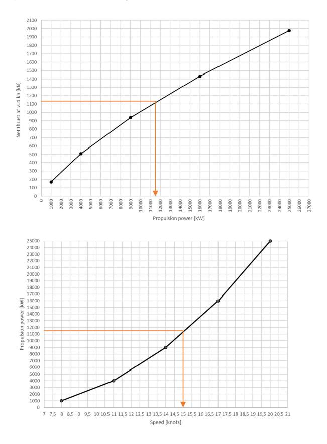
Now we simply need to calculate the ice resistance as a function of speed (two points, e.g. 0 m/s and 8 m/s) and the net thrust as a function of speed, and determine the intersection points. The values are collected to the following two tables:
