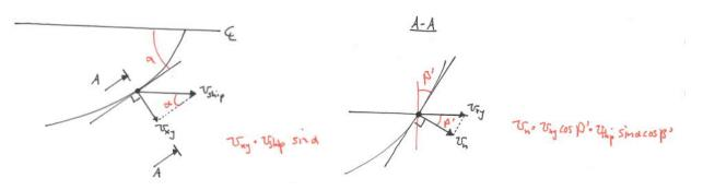
Since the owner is willing to accept an operational speed limitation of 9 knots (4.63 m/s), we can calculate the kinetic energy for each ice class (noting that  $V_n \approx 1.68 \frac{\text{m}}{\text{s}}$ ).
