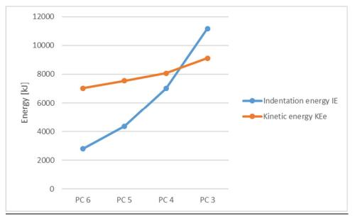
The graph indicates that if the operational speed limitation is 9 knots, the ice class must be PC 3 (or higher).
