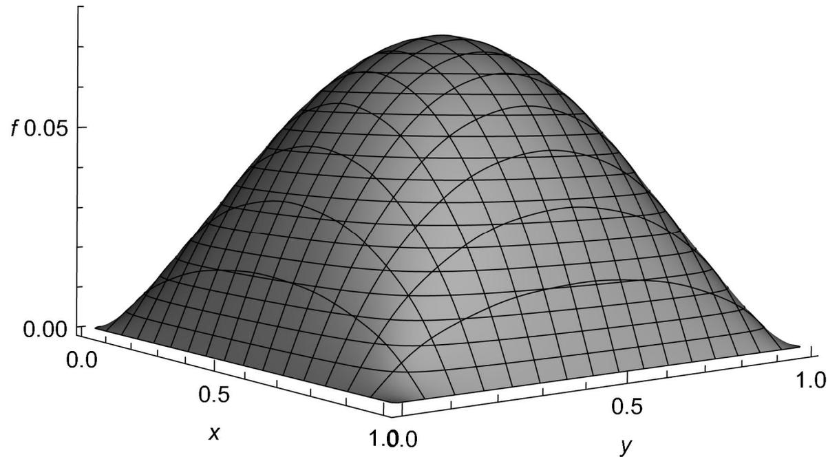
**EXAMPLE** Consider a rectangular drumhead of fixed edges, constant tightening  $S'$  (force per unit length) and density  $\rho t$  (per unit area). Find the frequencies of the free vibrations by using the double sine series trial solution
