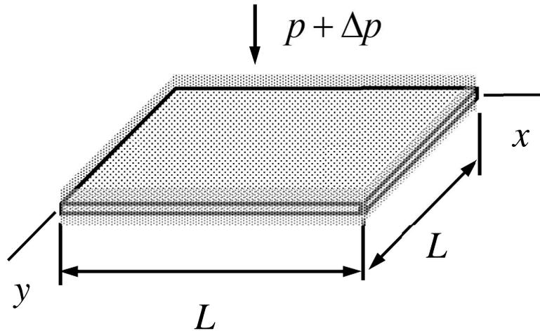
**Answer**  $w(x, y) = \sum_{k \in \{1,3,5,\dots\}} \sum_{l \in \{1,3,5,\dots\}} \frac{16}{\pi^4} \frac{\Delta p L^2}{S'} \frac{1}{kl(k^2 + l^2)} \sin(k\pi \frac{x}{L}) \sin(l\pi \frac{y}{L})$
