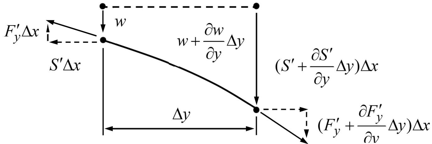
The tightening  $S'_x$  and  $S'_y$  (force per unit length) in the  $x$  – and  $y$  –directions may differ, in principle. Let us consider the isotropic case  $S'_x = S'_y = S'$ . As material elements are assumed to move only in the transverse direction, equations of motions in the horizontal directions become
