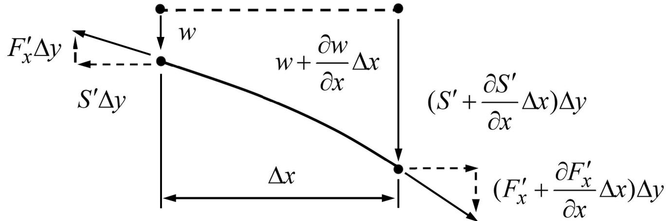
**Equation of motion**  $S' \left( \frac{\partial^2 w}{\partial x^2} + \frac{\partial^2 w}{\partial y^2} \right) + f' = m' \frac{\partial^2 w}{\partial t^2} \quad (x, y) \in \Omega \quad t > 0,$
