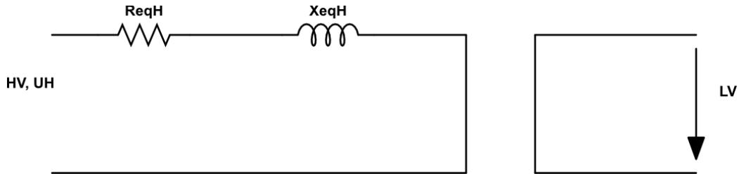
$$P_{sc} = R_{eqH} I_H^2 \Rightarrow R_{eqH} = \frac{P_{sc}}{I_H^2} = 0.18\Omega$$
