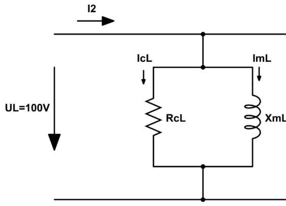
$$P_0 = I_{cL}^2 R_{cL} = \frac{U_{cL}^2}{R_{cL}} \Rightarrow R_{cL} = \frac{U_{cL}^2}{P_0} = 25\Omega$$
