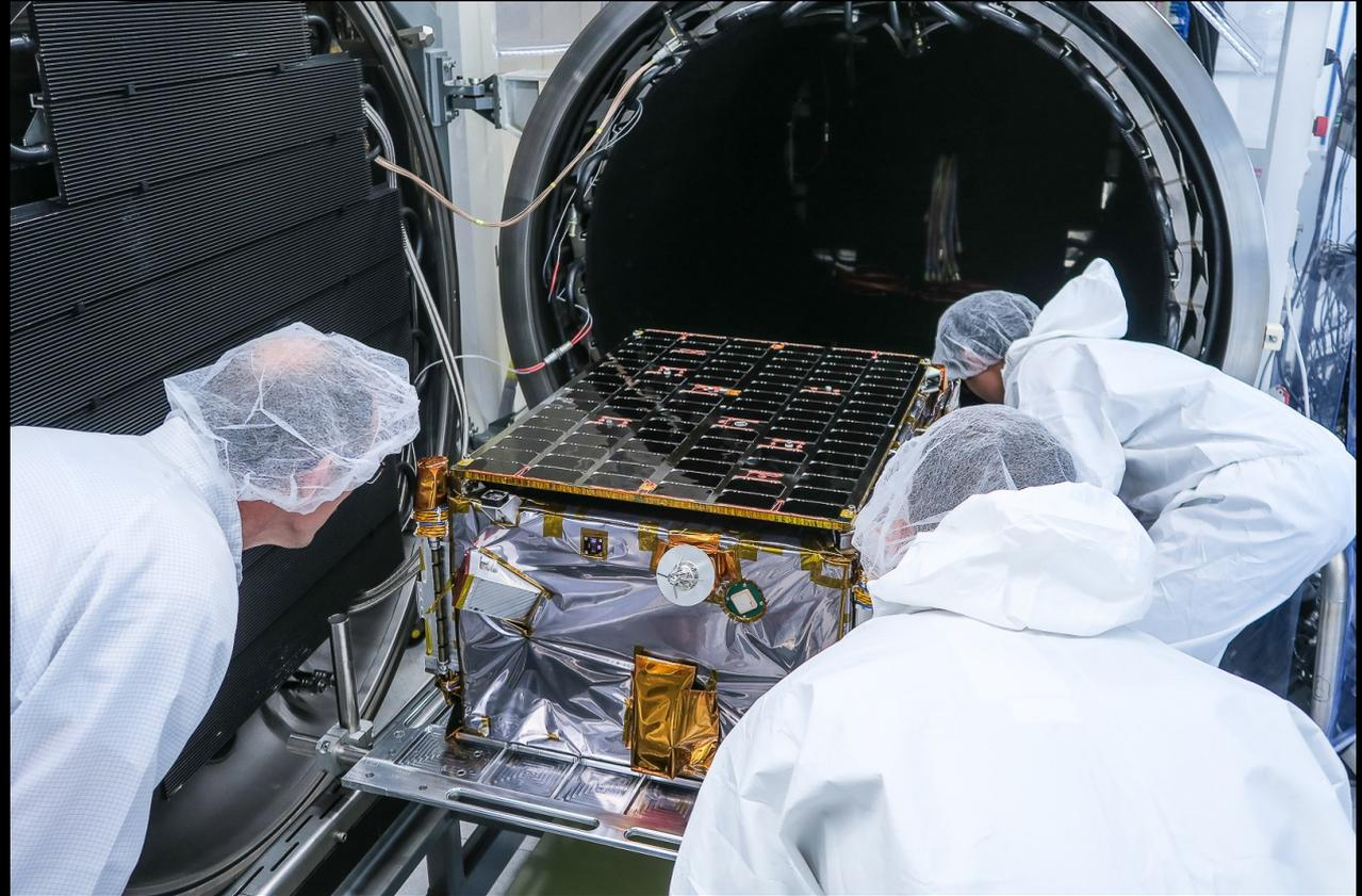
*ICEYE X1 satellite thermal vacuum tests in Germany 2017*
