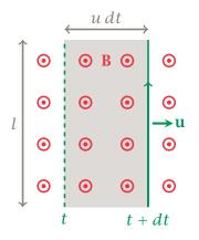
In time dt, the conductor sweeps the area
