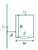
A time-varying current  $i_1$  in a long straight conductor induce a current  $i_2$  in a nearby rectangular loop. The resistance of the loop is R and the dimensions are given in the figure. Assume that  $di_1/dt > 0$  is given and derive  $i_2$ .
