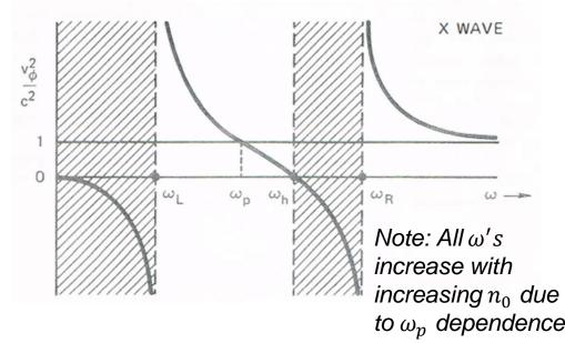
The resonance and cut-off frequencies divide the dispersion diagram into propagation and non-propagation zones.
