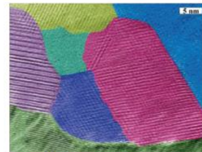
ZT~1.4 @ 373 K bulk – fine grain p-type, (Bi,Sb) 2 Te 3 [15 authors, BC/MIT/GMZ, 2008]
