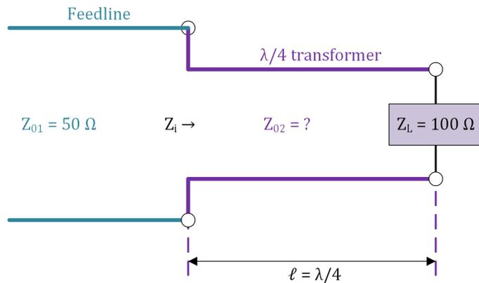
A  $50 \Omega$  lossless transmission line is to be matched to a resistive load impedance with  $Z_L = 100 \Omega$  via a quarter wave section as shown in the figure thereby eliminating reflections along the feedline. Find the characteristic impedance of the quarter wave transformer
