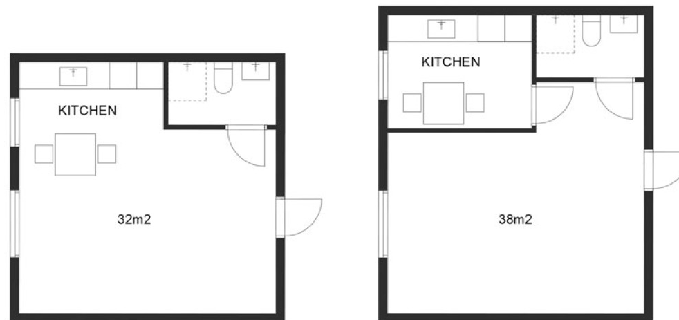
Figure 8. Floor plan diagrams of one-room apartments that illustrate the difference between kitchen types (open plan kitchen and separate kitchen).
