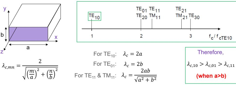
For rectangular waveguides, when a>b, the longest  $\lambda_c$  and the lowest cutoff frequency exist for TE<sub>10</sub> mode!!!
