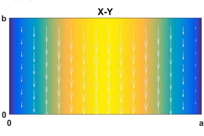
Electric field in the vertical axis is constant which corresponds to m = 0 (not sinusoid)
