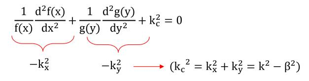
Decoupling to two 1-D wave equations
