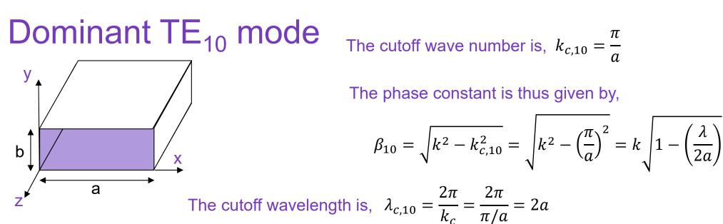
(the waveguide has to be at least greater than half of the wavelength in order for the wave to propagate)
