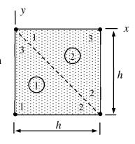
Derive the shape functions of the triangle elements 1 and 2 shown in the figure in terms of the (material) xy – coordinates.
