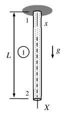
Finding the displacement of the free end follows the usual lines. Here,  $f_x = \rho g A$ ,  $u_{x1} = u_{X1} = 0$ , and  $u_{x2} = u_{X2}$
