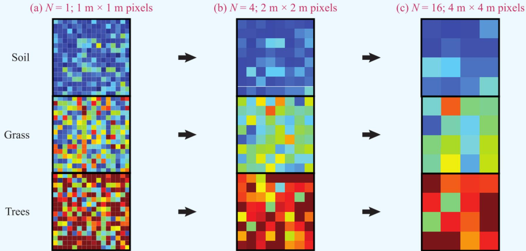
**Figure 5-21:** Simulated amplitude images of three distributed targets: trees with  $\sigma_t^0 = 36 \text{ m}^2/\text{m}^2$ , grass with  $\sigma_g^0 = 16 \text{ m}^2/\text{m}^2$ , and soil with  $\sigma_s^0 = 4 \text{ m}^2/\text{m}^2$ . Averaging multiple pixels trades off spatial resolution for improved radiometric resolution (less pixel-to-pixel variation).
