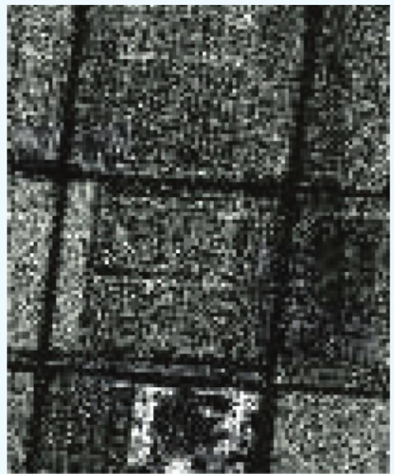
**Figure 5-13:** Image speckle refers to the pixel-to-pixel variation of image tone. This is a 1 m × 1 m resolution Ku-band SAR image of an agricultural area [Sandia National Lab].
