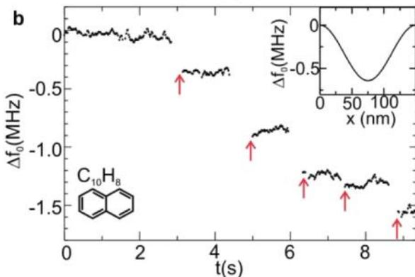
Monitor changes in resonance frequency as single molecules are absorbed.
