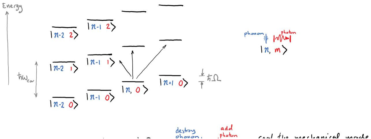
Transitions energy  $\hbar\omega_{\text{cav}} - \hbar\Omega$
