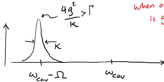
When optical damping rate is greater than mechanical damping ( $\frac{4g^2}{k} > \Gamma$ ) then we are effectively cooling the drum. The sideband linewidth depends on K (energy leaving via the optical cavity)
