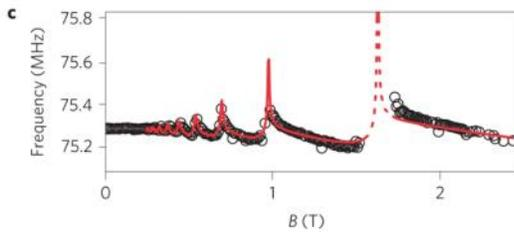
suspended graphene sheet is resonating at 75 MHz. The filling of Landau levels can be detected in the mechanical resonance.
