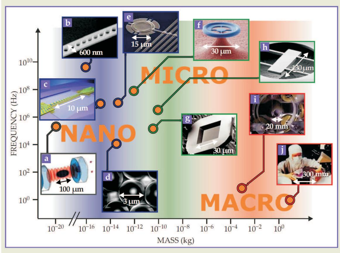
FIG. 1: Nanomechanical systems: (a) ultracold atoms in a cavity (b,c) optical photonic waveguides with mechanical oscillation frequencies (d) microspheres (e) metallic membranes (f) microtoroidal waveguides (g) microscale membranes (h) microscale devices, and (i,j) macroscopic resonators. Figure from Ref. [2].
