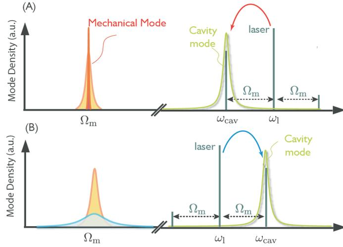
FIG. 5: (A) Amplification (laser is blue-detuned with respect to the cavity) and (B) cooling (laser is red-detuned with respect to the cavity). Scattering from the laser into the cavity is enhanced, leading to the amplification (suppressing of the anti-Stokes process and enhancing the Stokes process) and cooling (suppressing the Stokes processes and enhancing the anti-Stokes processes). Figure from Ref.[3].
