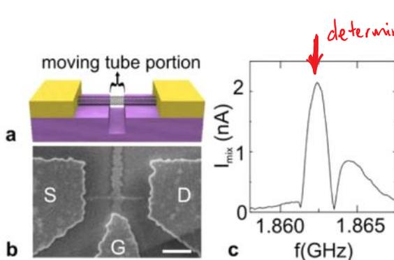
determine mechanical resonance from jump in  $I_{mix}$  when CNT motion is large (significant modulation of  $G$ )
