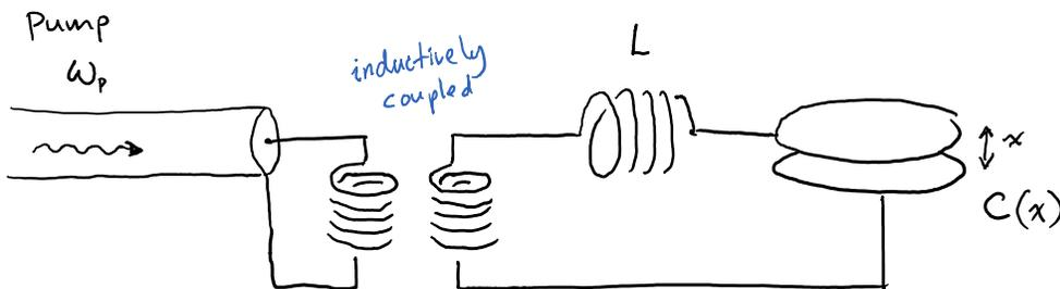
The LC resonator  $\equiv$  cavity
