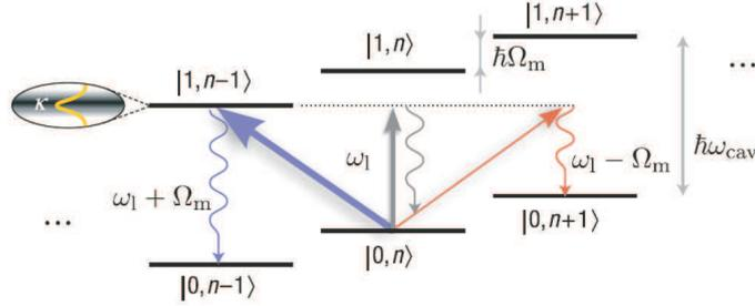
FIG. 4: Diagram of transitions. The cavity, if it is higher in frequency than the laser, enhances the transitions that result in loss of phonons from the mechanical resonator. Figure from Ref. [3].
