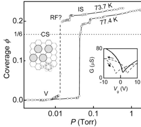
Fig. 3 Adsorption of Kr on device YB3, showing first-order phase transitions. (The 73.7 K isotherm has in-
