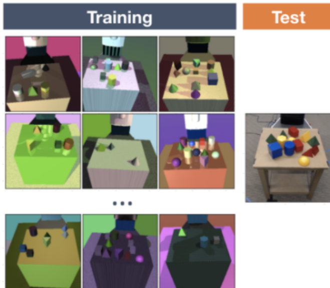
Figure 2. Randomized images are created through visual randomization on which model is trained to be able to transfer to real non-randomized images[15].
