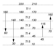
The heat content for the hot streams is calculated from  $\dot{m} \cdot cp(T_{start} - T_{target})$  and  $\dot{m} \cdot cp(T_{target} - T_{start})$  for the cold streams..<sup>1</sup>
