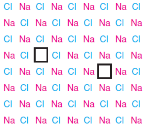
Figure 2.2 2D representation of a Schottky defect with cation and anion vacancies.
