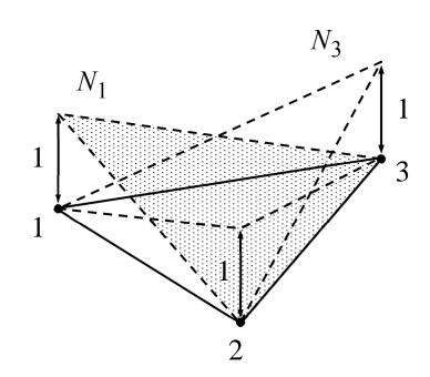
Triangle element is the simplest element in two dimensions. Division of any 2D domain into triangles is always possible, which makes the element quite useful.
