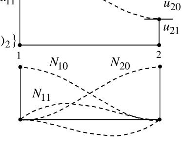
In xz -plane bending  $u = u_z$ ,  $du / dx = -\theta_y$  and in xy -plane bending  $u = u_y$ ,  $du / dx = \theta_z$ .
