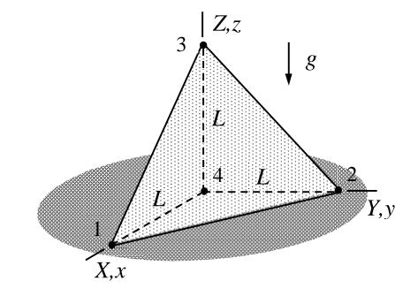
• Linear shape functions can be deduced directly from the figure  $N_1 = x/L$ ,  $N_2 = y/L$ ,  $N_3 = z/L$ , and  $N_4 = 1 - x/L - y/L - z/L$ . However, only the shape function of node 3 is needed as the other nodes are fixed. Approximations to the displacement components are
