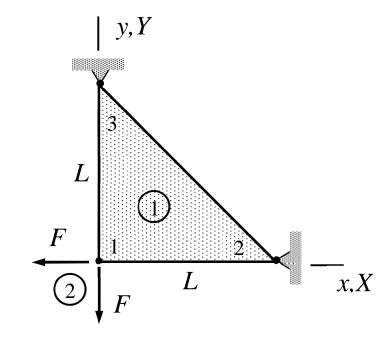
• Nodes 2 are 3 are fixed and the non-zero displacement components are  $u_{X1}$  and  $u_{Y1}$ . Linear shape functions  $N_1 = (L - x - y)/L$ ,  $N_2 = x/L$  and  $N_3 = y/L$  are easy to deduce from the figure. Therefore
