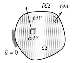
Although the two representations are equivalent, principle of virtual work combines the equations in a way which is the key for multiple important applications in mechanics. Finite element method is just one of them.
