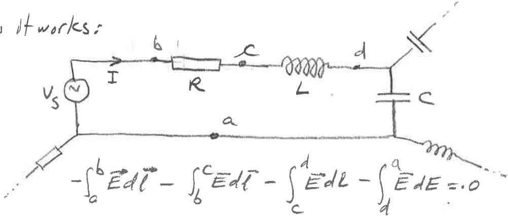
$$\text{or } V_s(t) - R I(t) - L \frac{dI(t)}{dt} - \frac{1}{C} \int_a^t dC I(z) = 0$$
