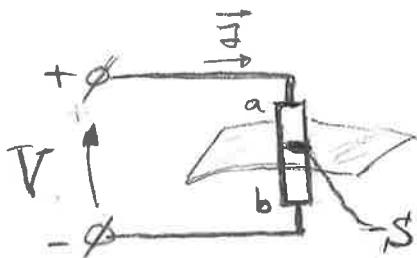
$$V = V_a - V_b = - \int_b^a \vec{E} \cdot d\vec{l} = \int_a^b \frac{\sigma}{S} \vec{J} \cdot d\vec{l}$$
