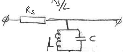
$$Z_p = \frac{i\omega L \cdot \frac{1}{i\omega C}}{i\omega L + \frac{1}{i\omega C}} = \frac{i\omega L}{1 - \omega^2 LC}$$
