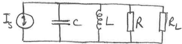
$$Q_L = \left( \frac{1}{R} + \frac{1}{R_L} \right) \sqrt{\frac{C}{L}} = \text{loaded } Q$$
