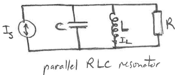
$$Z(\omega) = \frac{1}{G + i \frac{C}{\omega} (\omega^2 - \omega_0^2)} = \frac{1}{Y(\omega)}$$
