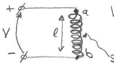
$$V = V_{ab} = V_a - V_b = - \int_b^a \vec{E} d\vec{l} = \iint_S \frac{d\vec{B}(t)}{dt} d\vec{s} = L \frac{dI}{dt}$$
