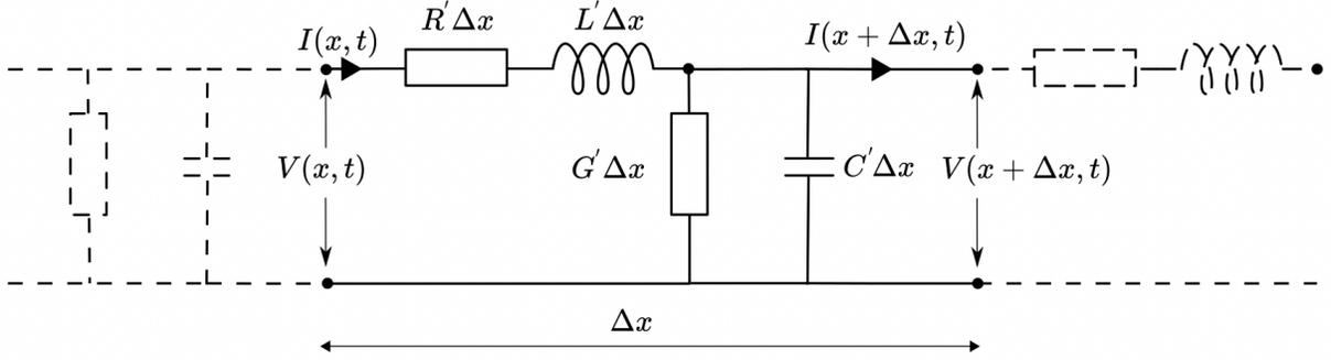
$R', L', G', C'$  = resistance, inductance, conductance, capacitance per unit length.
