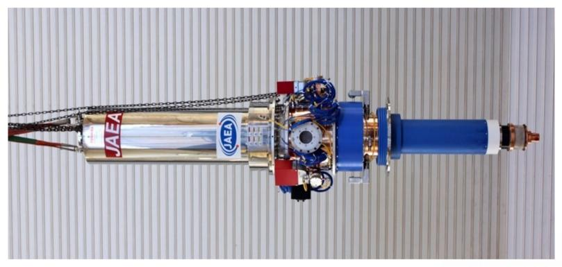
Each of ITER's 24 gyrotrons will generate a microwave beam over a thousand times more powerful than a traditional microwave oven. www.iter.org.
