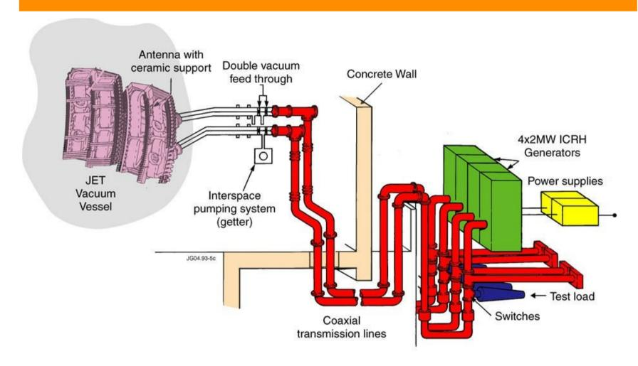
For practical reasons, antennas installed at low-field side ⇒ low-loss coaxial transmission lines to tokamak
