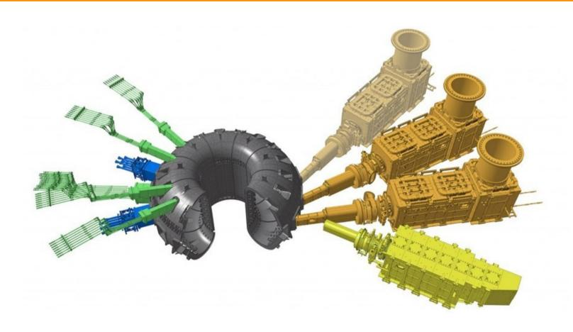
Neutral beam injection (right) and two sources of high-frequency electromagnetic waves—ion and electron cyclotron heating (left, blue and green launchers). www.iter.org.
