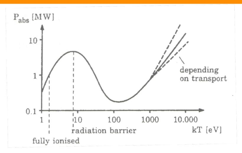
For medium-size tokamaks (e.g., ASDEX Upgrade) 1 MW is needed to fully ionize, and 5 MW to offset radiation
