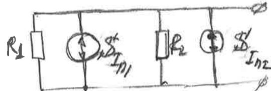
$$S_{I_m} = S_{I_{m1}} + S_{I_{m2}} \leftarrow \text{again uncorrelated fluctuations of current}$$
