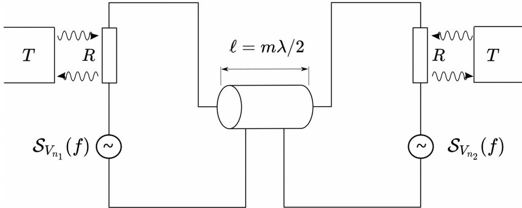
This time  $R_1 = R_2 = R$  but the connection is done through a TL (transmission line).
