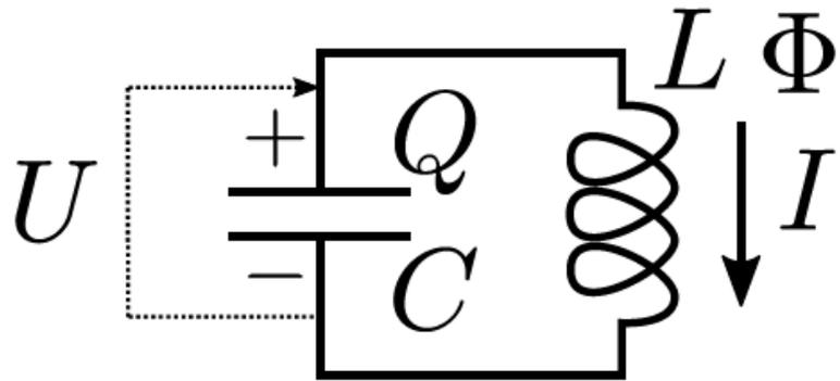
Figure 2: Superconducting LC oscillator.
