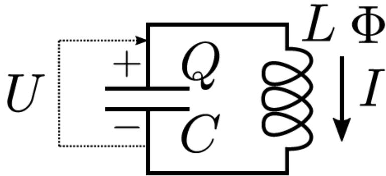
Figure 2: Superconducting LC oscillator.
