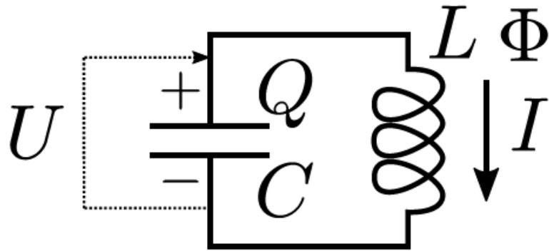
Figure 2: Superconducting LC oscillator.
