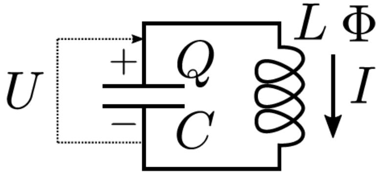
Figure 2: Superconducting LC oscillator.
