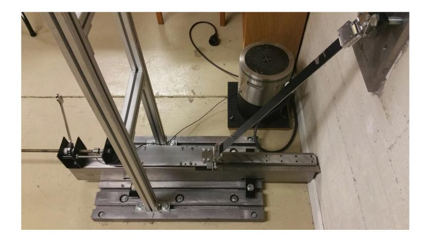
**Does**  $p_{cr} = \pi^2 \frac{EI}{(KL)^2}$  predict the buckling force within engineering accuracy?
