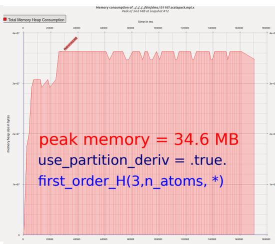
Figure 3.8: The memory profiles using valgrind are shown for DFT and three DFPT vibration keywords. It is clearly shown that the DFPT\_vibration\_reduce\_memory(28.4 MB) code just use nearly the same memory as DFT (28.0MB) calculation, while DFPT\_vibration(33.2 MB) and DFPT\_vibration\_with\_moving\_gird(34.6 MB) need higher memory because they stored matrix as (3,n\_atoms, \*).
