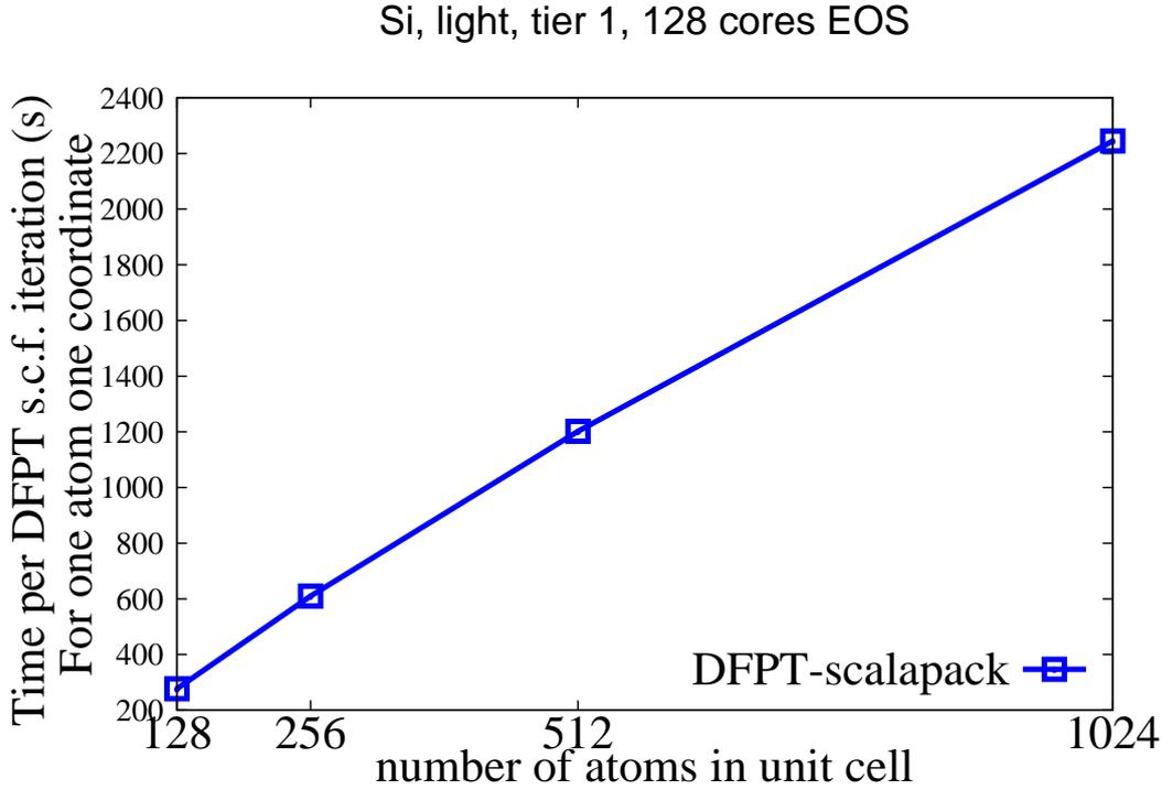
Figure 3.10: The CPU time per DFPT cycle as a function of the number of atoms in unit cell on 128 CPU cores.
