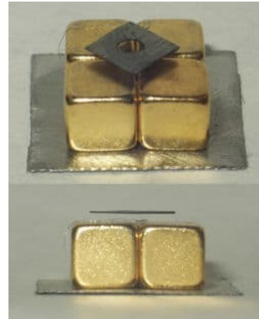
Pyrolytic carbon bar levitates above permanent magnet
