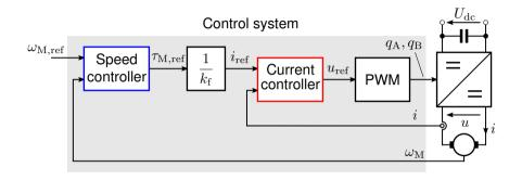
**Current controller:** Inner (faster) loop **Speed controller:** Outer (slower) loop
