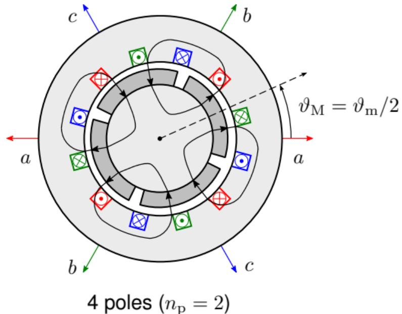
Electrical angular speed  $\omega_m = n_p \omega_M$  and electrical angle  $\vartheta_m = n_p \vartheta_M$
