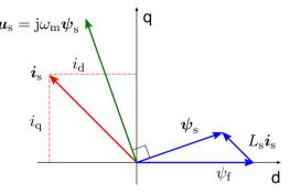
Above the base speed:  $i_{\rm d} < 0$  in order to reduce  $| \pmb{\psi}_{\rm s} |$
