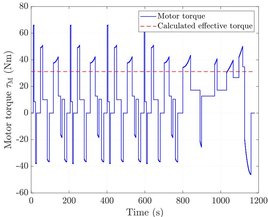
**Figure 3:** Motor torque (solid blue line) and the calculated effective torque (dashed red line) in an example case. It is to be noted that the calculated effective torque is not directly the root-mean-square value of the motor torque, because the motor is operating both in the full-field region and in the field-weakening region in this example (cf. Section 3.3).
