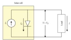
Figure: Model of the solar cell
