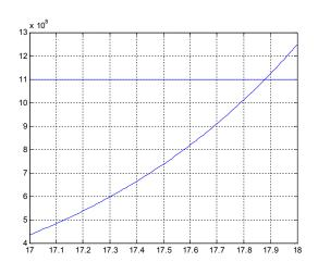
Based on the drawings, it can be concluded that at maximum power point  $\frac{V_{mp}}{V_T} \approx 17,88$ . Then the current of the maximum point is
