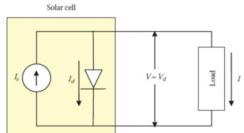
Figure: Model of the solar cell
