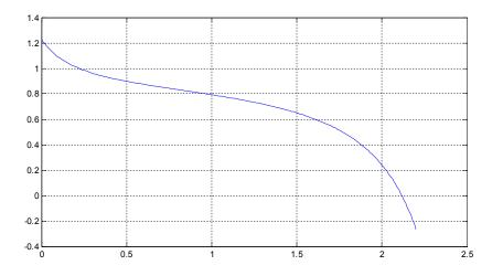
From the derivative and also from the power curve one can conclude that the maximum power point is around 2,1 A and voltage is then
