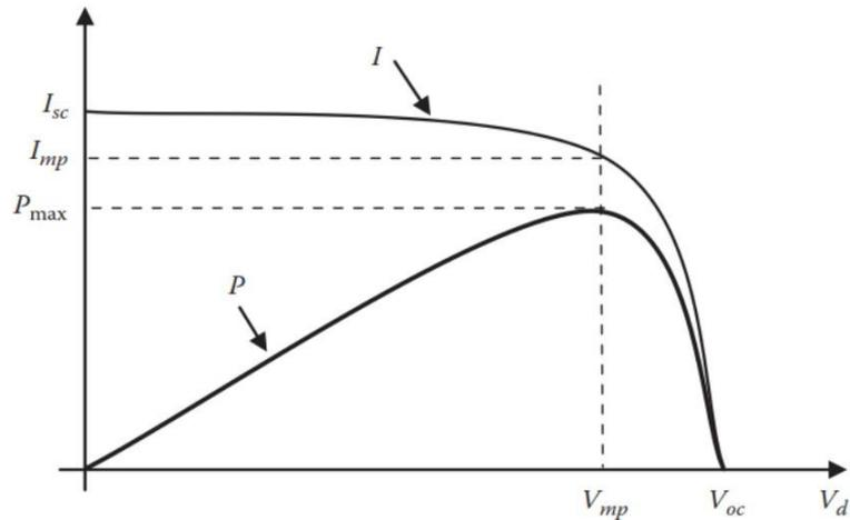
As can be seen from the above characteristics, there is a point at which the power is maximum for a specific voltage and a current value. If the cell operates at these specific values, the maximum power can be reached.
