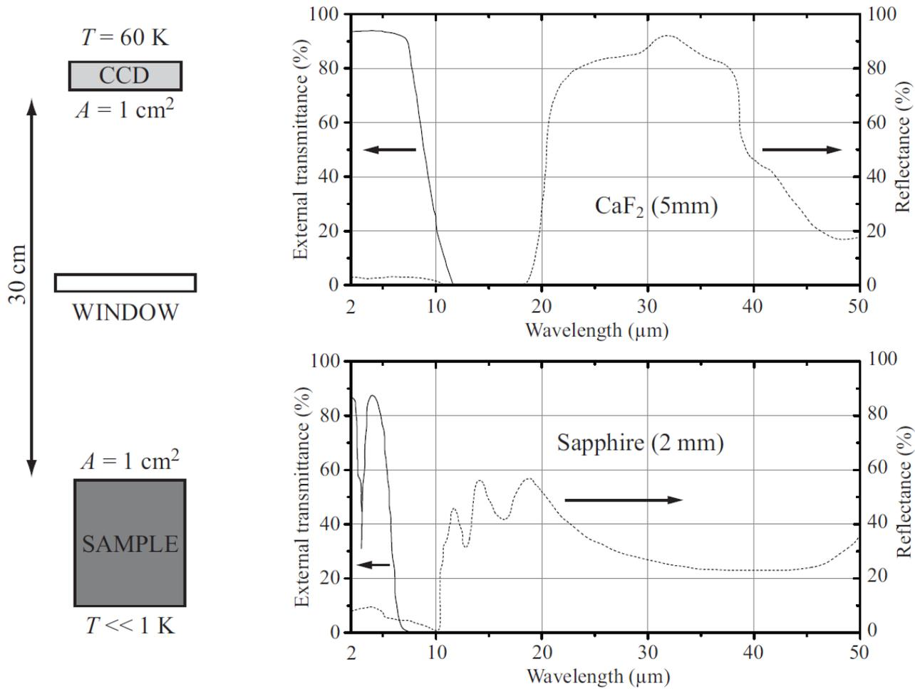
Figure 1: Schematic of the imaging setup and transmittance properties of CaF<sub>2</sub> and sapphire.
