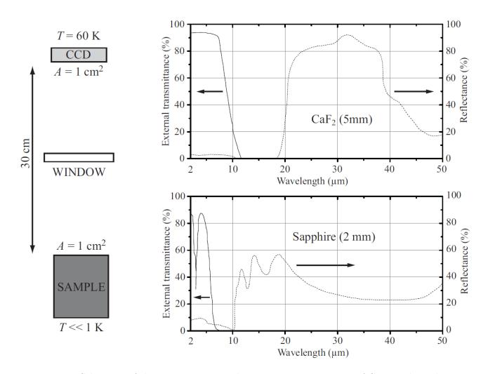
Figure 1: Schematic of the imaging setup and transmittance properties of  $CaF_2$  and sapphire.
