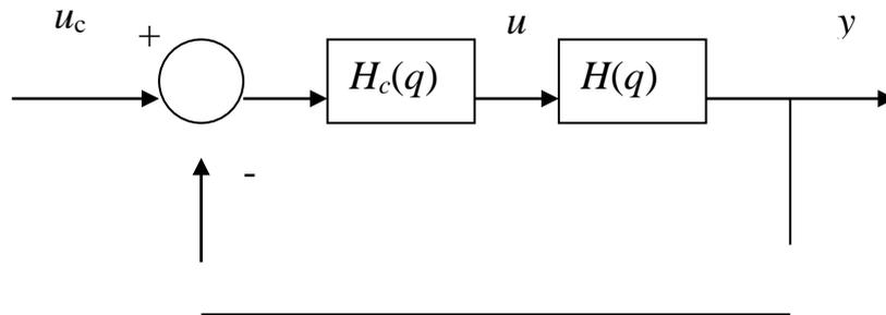
Assume that the sampling time is  $h$  and D/A-converter holds the control signal constant during the sampling period. The control algorithm is
