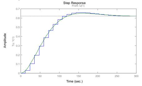
Note that in the above example the command ss2tf was used. Another, maybe more common way today would be to read the numerical values into matrix objects Phi, Gamma, C, D, and then write something like Gss=ss(Phi,Gamma,C,D,12); G=tf(Gss).
