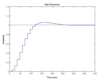
The steady state error is removed when the integrator was added to the controller.
