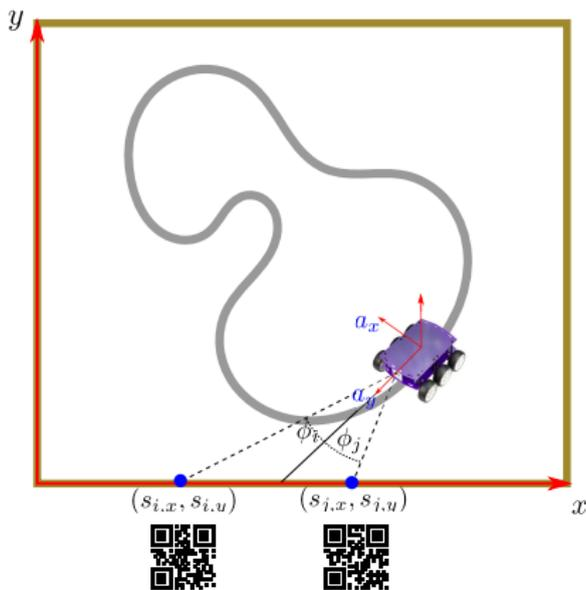
**Figure:** Illustration of the global coordinate system, QR-codes with known positions in global coordinate, and the robot local acceleration. When the robot camera heads to the  $y$  axis, the global angle of the robot equal to zero.
