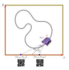
Figure: Illustration of the global coordinate system, QR-codes with known positions in global coordinate, and the robot local accerelation. When the robot camera heads to the y axis, the global angle of the robot equal to zero.
