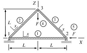
5. Determine the nodal displacements, when force *F* is acting on the structure as shown in the figure. The cross-sectional area of all the bars is *A* and the Young's modulus of the material is *E*. Use the principle of virtual work.
