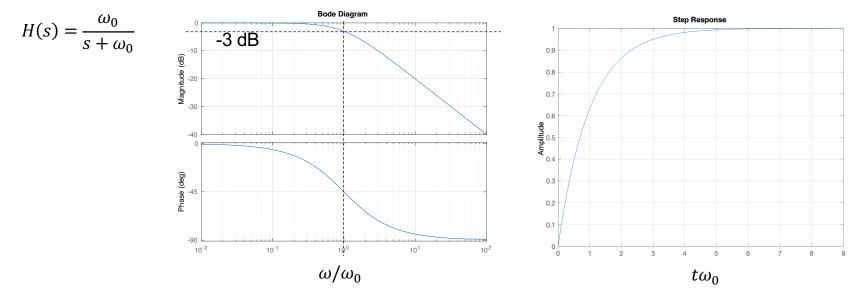
$\omega_0$  large => wide bandwith => fast response  $\omega_0$  small => narrow bandwith => slow response
