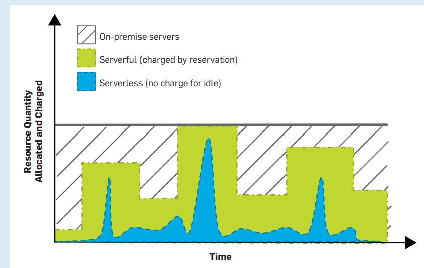
Figure 3. Serverless vs Serverful cloud computing: serverless users pay only for resources consumed, not for idle reserved capacity.
