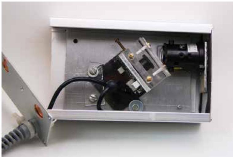
An image of a USB spectrometer (Source: USB Spectrometer. 2019)
